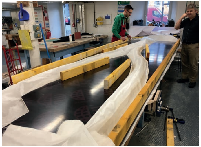
One half of the formwork for one of the trees.
