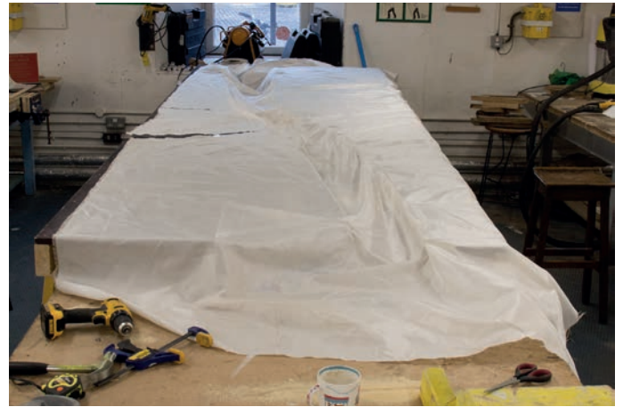
Fastening of fabric. The fabric was stapled all along edge of the cut-out shape.
