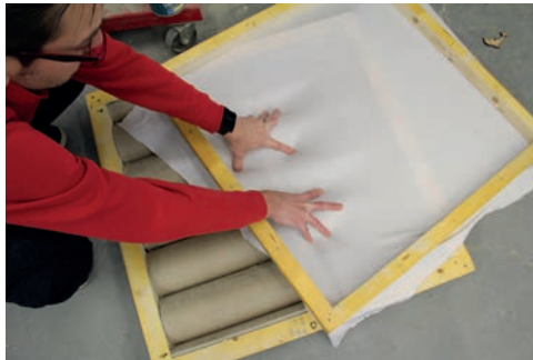
Before and after shot of a panel. The panel was made using a flexible fabric moulding around cardboard tubes.
