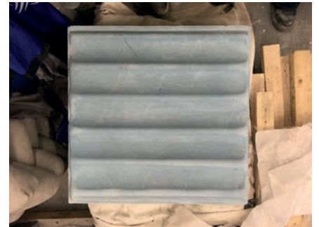
Before and after shot of a panel. The panel was made using a flexible fabric moulding around cardboard tubes.
